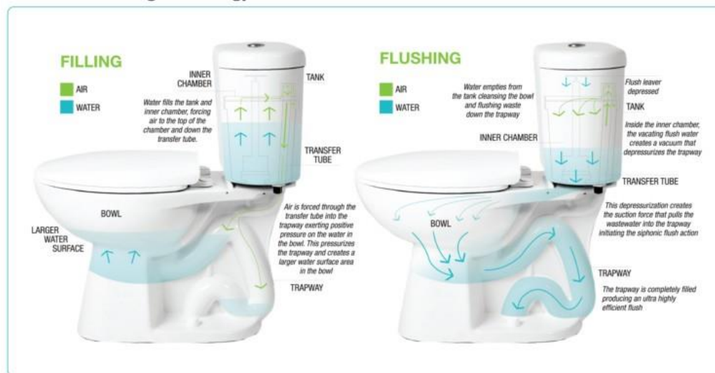
Figure 47 Principle of the Stealth Flushing technology – a vacuum assist toilet flushing system (Niagara conservations, 2013)
